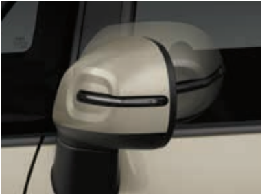
Door-lock-system-connected folding outside mirror*
