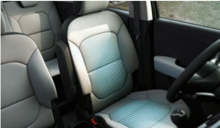
Ventilated driver's seat (linked with Kia Connect)* A fan embedded in the seat provides ventilation to create a comfortable driving environment.
